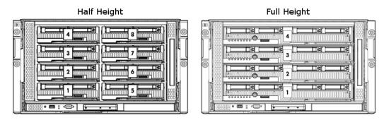
The number of fans in the enclosure influences the placement of the server blades. Use the following table and the numbering scheme in Figure 1-8 to determine the placement of the server blades in the enclosure, based on the number of fans.
